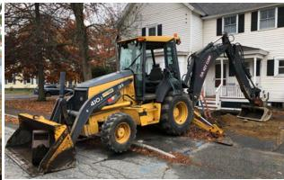
GETTING TO THE BOTTOM OF IT. Repairing a root-clogged sewer line at the Parsonage required the heavy equipment of local firm DR Key, which upgraded the old clay pipe with new PVC line.
